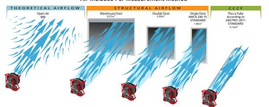
During the ventilation process, airflow from the fan will create large amounts on entrained air. Entrained air is the natural effect from the high velocity airflow creating friction with the air next to it, thereby pulling the air into the flow path. While measuring airlfow, entrained air that goes through the opening must be included in the airflow calculation to reflect realistic ventilation obtained by the fan.
