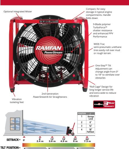
Note: Output changes as setback from the opening changes. Single door airflow is per AMCA 240-6 testing. This data derives from 0° static pressure. Test results from fan set back 5.5m at 12° tilt and 3,684 rpm. Real world results will be substantially reduced by structure back-pressure.
